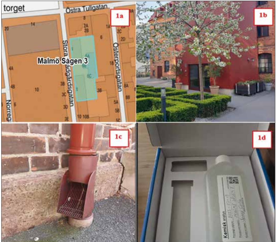
Figure 1. Figure 1a shows the property designation, Sagen 3 in Malmö, Sweden. Figure 1b shows the building at Sagen 3. Figure 1c shows a detailed photo of the gutter where sampling took place. Figure 1d displays the sampling container and, consignment box. Photo by Sonny Colin.
