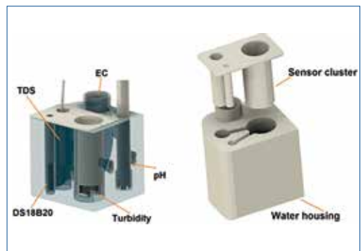
Figure 2. To the left, complete assembly of sensor body and sensor cluster. To the right, sensor cluster and water housing separated (sensor cluster and holder, own illustration, but with DS18B20 sensor by Medina, 2019; TDS sensor by Suresh, 2021; turbidity sensor by Arrieta, 2019 and pH sensor by Happysoft, 2018).
